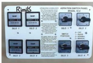
The RIMIK switch panel for switching control modes for multiple silos.
